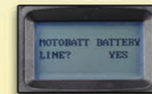
4 BATTERY TYPE AVAILABLE TO TEST: A.REGULAR LIQUID B.AGM FLAT PLATE C.AGM SPIRAL D.VRLA/GEL
