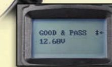
5 TEST RESULTS: A.GOOD & PASS B.GOOD & RECHARGE C.RECHARGE & RETEST D.BAD & REPLACE E.BAD CELL & REPLACE
